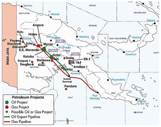
Figure IX.11.7. Location map of main oil and gas fields of PNG (PNG Chamber of Mines and Petroleum).
