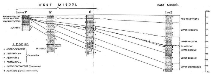
Figure VIII.2.3. W-E stratigraphic cross-section across Misool, showing 'mid-Oligocene' unconformity, most pronounced in West Misool (Roggeveen 1939 in Van Bemmelen, 1949).
