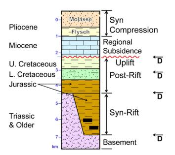
Figure IX.11.4. Diagrammatic stratigraphy of Mesozoic- Tertiary of Papua- New Guinea foldbelt, with approximate thicknesses. (Juha field; Hanani et al. (2016). Mesozoic rift- passive margin sequence, Upper Cretaceous uplift event, Plio-Pleistocene syn-compressional flysch and molasse. D= detachment surfaces.
